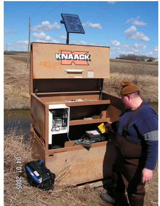
Automated water samplers allow RCRC to be a leader in water quality testing and reporting. Here Watershed Technician, Doug Goodrich, sets up a sampler for the 2005 sampling season.
